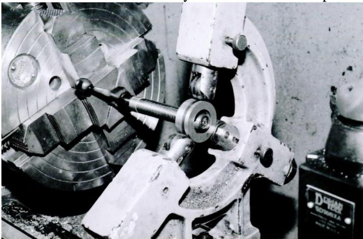
Photo #7. Use great care in facing off the rear faces of the bolt locking lugs. Select a left-side facing tool-bit having a generous 0.060-inch tip radius, and fair the facing cut into the factory fillet at the bottoms of the lugs.
