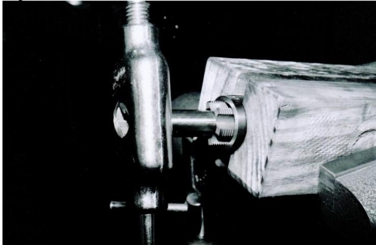
the threads in these receivers. We had a similar piloted tap made at +0.015-inch, but only used it once in over 200 applications. The piloted tap must be rather carefully started *in-phase* with what remains of the original factory threads. [Photo #3 shows the set-up for this step]. Note that this strongly (doubly) piloted tap does not, and indeed cannot, merely follow the miss-
