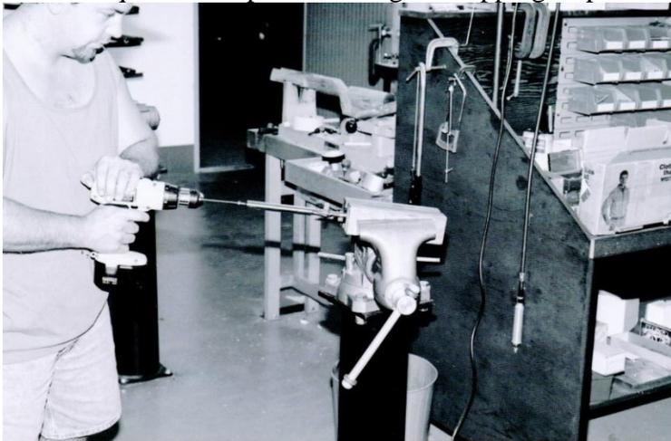
a pair of 0.7050-inch pilots and make a “clean-up pass” through the action from the other direction. This reverse pass reduces the reamer marks in the boltway and also reduces the hand deburring that will be done later. [Photo #2 shows this reaming set-up].
