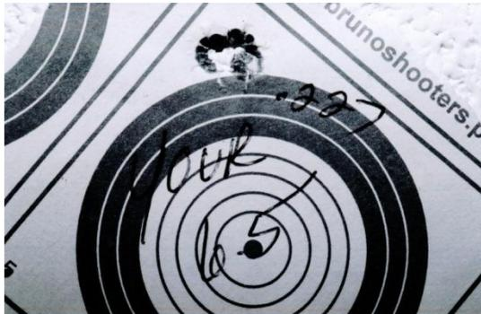
complete rifles and test them in our indoor 105-yard instrumented test range attached to our shop. Photo #11 shows a single five-shot group recently fired (in 2003) by two different shooters using two slightly different loads in 6.5mm-284 Norma. It was fired using our prototype tactical rifle [Photo # 12] made by blueprinting a Remington 25-06 Sendero and converting it to 6.5-284 Norma using a stainless steel Krieger 8.5-inch twist
