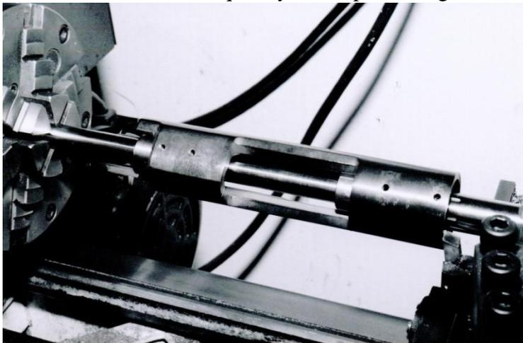
all of the factory threads have been re-cut, the tap itself will be well down inside the front ring of the receiver by the time the tap becomes too tight to turn by hand. At this point, the piloted tap can be used as a mandrel to hold the receiver squarely in any available lathe for minimally facing off the front surface of the
