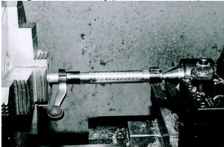
metal to the action in the truing process. The rear of the bolt is held in a four-jaw chuck using a shop-made threaded mandrel. The bolt-engaging threads of the mandrel used for holding the rear of the bolt body are purposely made to be a loose fit so that the orientation of the bolt can be slightly adjusted without stressing the bolt. The front of the bolt is held by the tailstock
