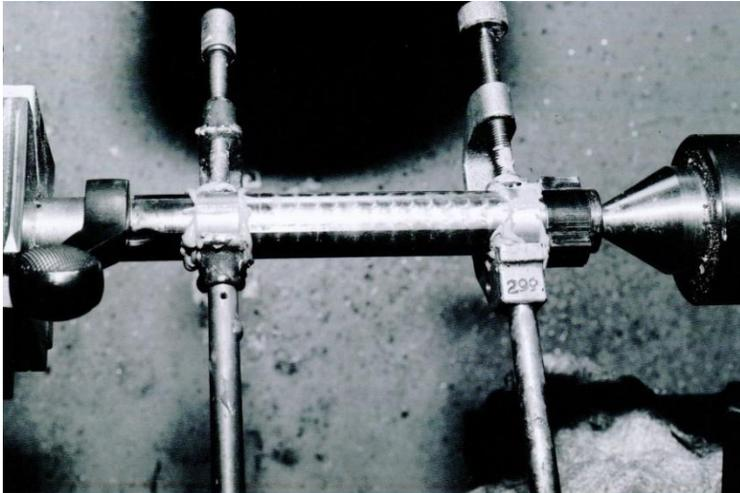
two sleeves are turned to 0.7049-inch OD and the rear faces of the recoil lugs are minimally faced off square, being careful not to touch the radius at the bottom of the lugs. Then, if the geometry of your steady-rest rollers permits, you can run them directly upon the front sleeve. With some lathes like our Nardini, we install a sacrificial sleeve over the bolt lugs, held in place with
