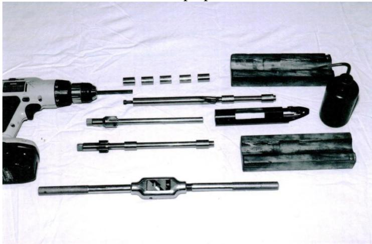
be sleeved, front and rear, with two stainless steel rings of an outside diameter (OD) to match the ID of the trued boltway. The axis of the two installed bolt sleeves is constrained by its set-up in the lathe to pass through the center of the firing pin hole in the bolt face. The critical rear faces of the bolt locking lugs are faced off by the minimum amount to make them perpendicular to the
