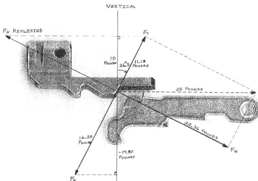
because *only the normal force component  $F_n$ , and neither of the two tangential forces  $F_t$  or  $F_f$ , is “reflected” back into the cocking piece by the angled contact face of the fixed (supported) sear.*
