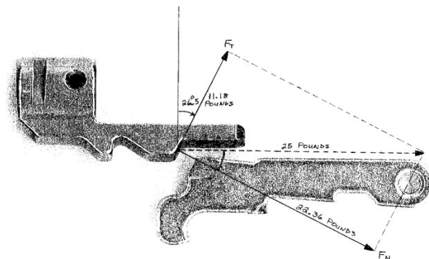
**degrees**, and  $F_t$  tangent to the sear contact surface, as diagrammed in Figure 3. As the diagram shows, these two rectangular force components ( $F_n$  and  $F_t$ ) would *vector sum* to equal exactly the original imposed **25-pound** spring force  $F$ . Just as the spring force  $F$  can be *replaced* by its component forces  $F_n$  and  $F_t$ , we can also replace the reaction force (**minus  $F$** ) of the
