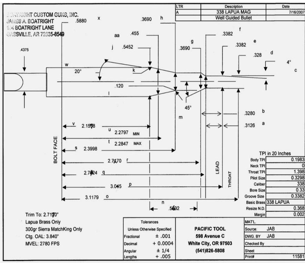
**Notes:** Dimensions **n**, **q**, **r**, and the “Trim-to” Length were each increased by **0.010-inch** after experience with the first two rifles chambered with this reamer. As of Sept 16, 2009, the dimensions are to be:
